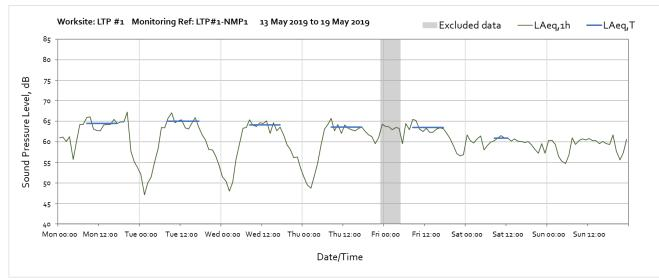
Note: High noise levels in the night of the 16<sup>th</sup> were due to temporary closure of the M25 and high levels of road traffic noise due to diverted traffic along the A412. Measured noise levels were not representative of HS2 construction noise during this period.
