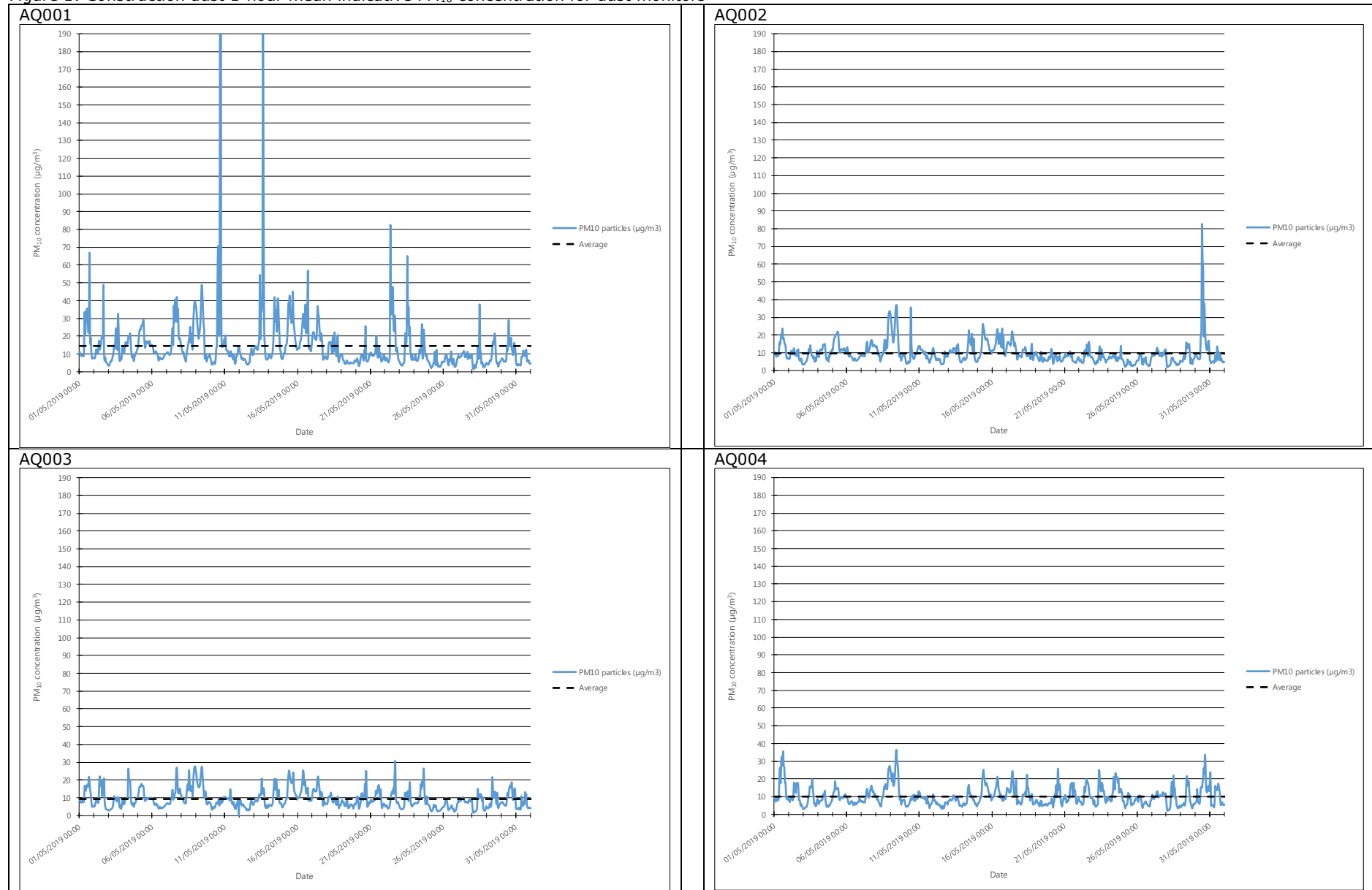
Figure 1: Construction dust 1-hour mean indicative PM 10 concentration for dust monitors
