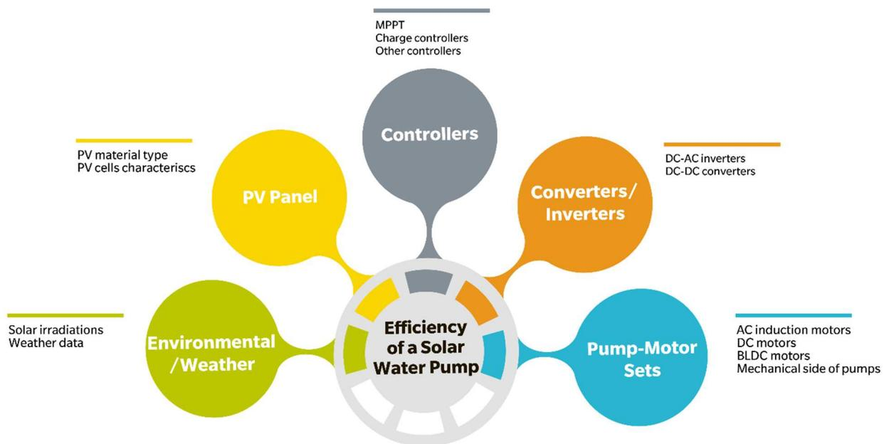
Figure 5: Key factors influencing the efficiency and performance of a solar water pump.
