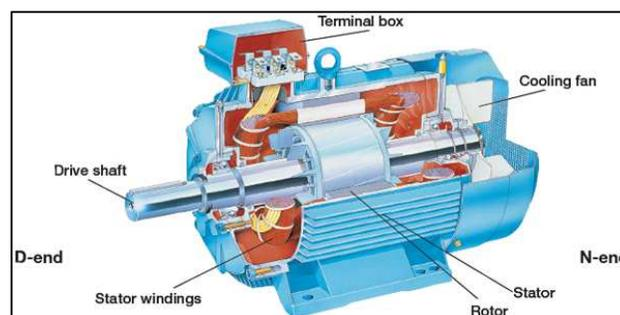
Figure 12: Key components of an AC induction motor.<sup>61</sup>
