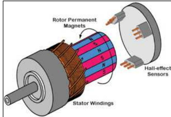
Figure 13: BLDC motor construction.<sup>65</sup>
