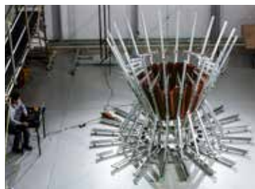
Oxford Space Systems' origami-inspired folding satellite. © Adam Gasson
