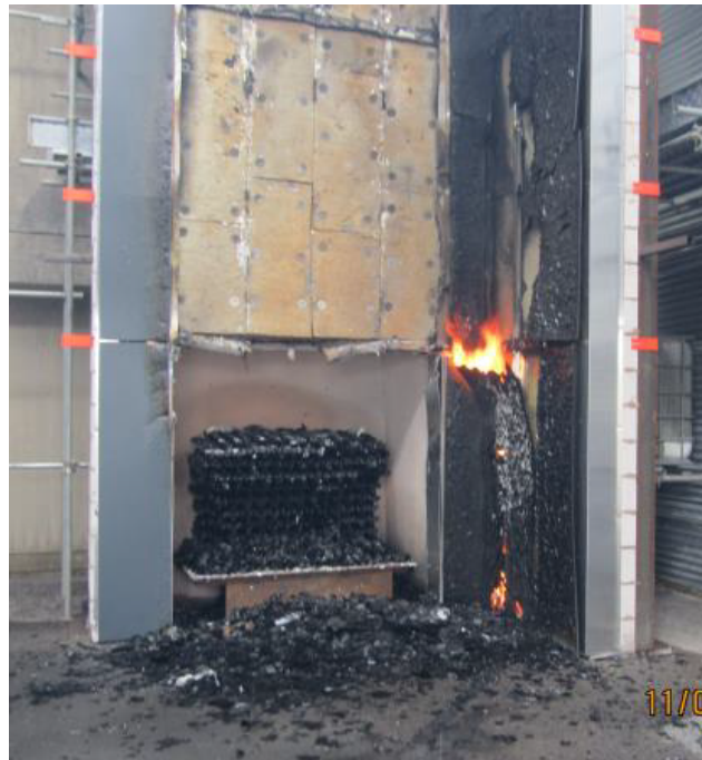
Figure 15 – Flames on panel 13 immediately before test end
