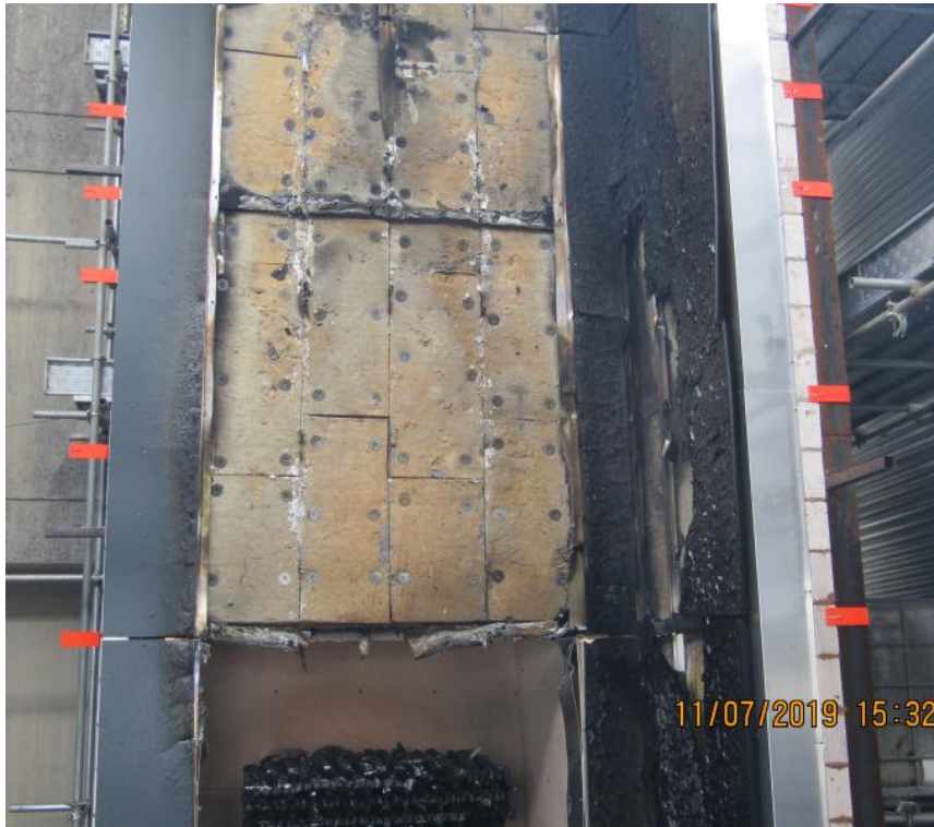
Figure 21 – Area directly above combustion chamber post test
