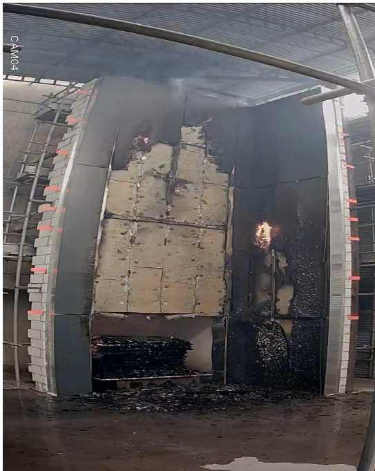
Figure 14 – Residual burning on panels 2, 3 and 10 following extinguishment of the crib
