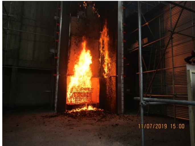
Figure 13 – Test wall and debris in front of wall prior to extinguishment of the crib. (29 minutes 50 seconds from ignition)
