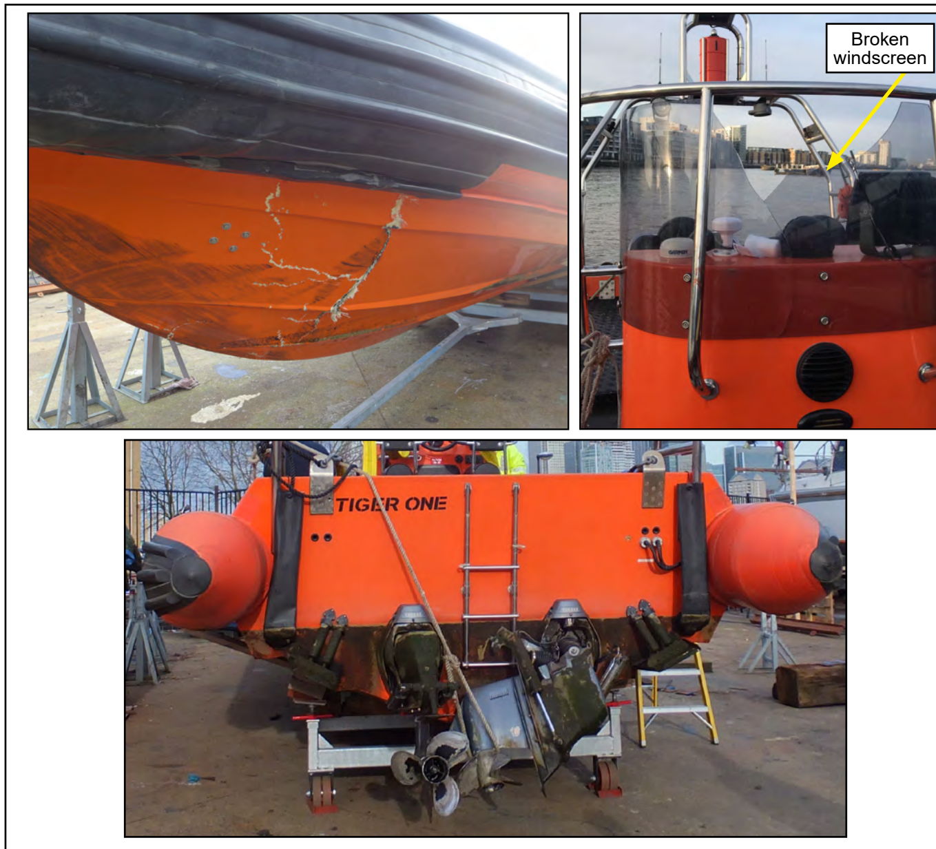
Figure 4: Damage to bow, windscreen and stern drive
