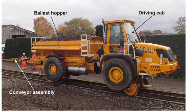
Figure 3: The ballast distributor road-rail vehicle
