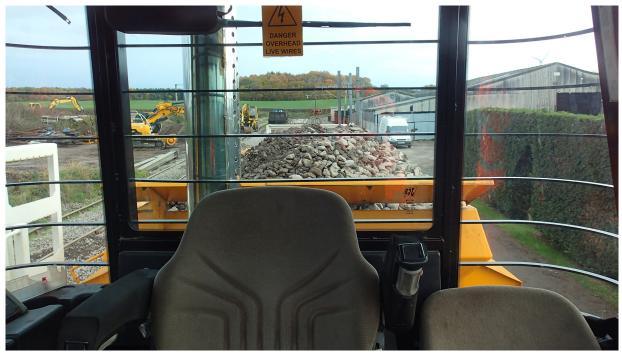
Figure 10: Driver's and second person's seats in the ballast distributor cab
