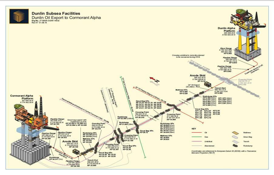
Figure 1-4: Dunlin Alpha to Cormorant Alpha pipeline (PL5)
