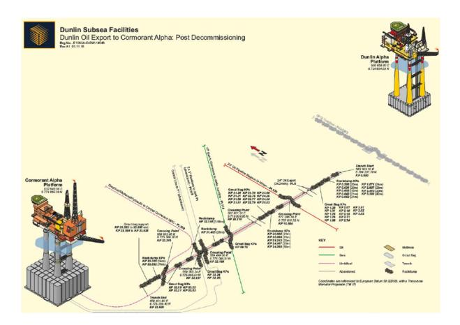
Figure 6-2: Dunlin Alpha to Cormorant Alpha pipeline (PL5) - Post Decommissioning Overview
