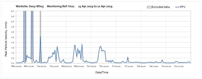
Note: High vibration levels at 08:00 and, 15:00 on Monday 15<sup>th</sup> and at 23:00 on Tuesday 16<sup>th</sup> of April were due to local disturbance of the vibration monitor and are not representative of HS2 vibration levels.
