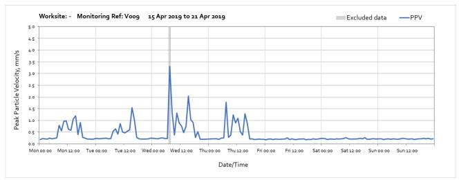
Note: High vibration levels at 07:00 on Wednesday 17<sup>th</sup> of April were due to local disturbance of the vibration monitor and are not representative of HS2 vibration levels.
