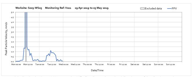
Note - High vibration levels at 10:00 on Monday  $29^{th}$  of April were due to local disturbance of the vibration monitor and are not representative of HS2 vibration levels.
