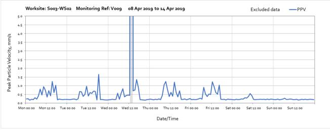
Note: High vibration levels at 12:00 on Thursday 10<sup>th</sup> of April were due to local disturbance of the vibration monitor and are not representative of HS2 vibration levels.
