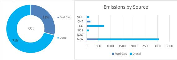
The primary source of  $CO_2$  emissions from Foinaven FPSO is diesel which supplies power generation. Note the field operator, BP, is responsible for managing the flare consent and EU ETS permit associated with the Foinaven fields and therefore flare data is not included here.
