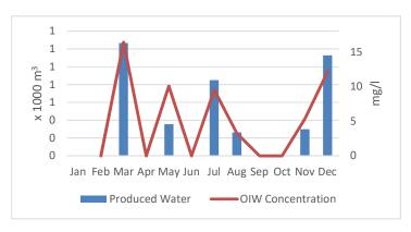
The average OIW concentration for the period was 12 mg/l, below the permitted 30 mg/l limit. A produced water volume of 4,164 m³ and 50 kg of oil was discharged during the period.
