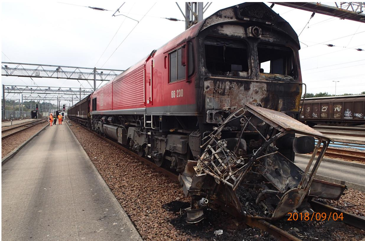
Figure 11: Image of locomotive and damaged buggy following accident. Concrete walkways run between each siding and are used for the inspection of trains.
