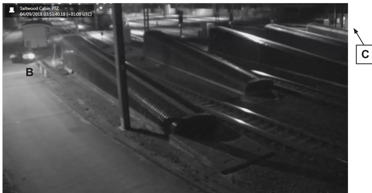
Figure 10: CCTV still image showing ramps and west end level crossing. Locations B and C are as marked on figure 8. The buggy is visible at location B, approaching the west end level crossing. The collision occurred just outside of the camera's field of view at location C.
