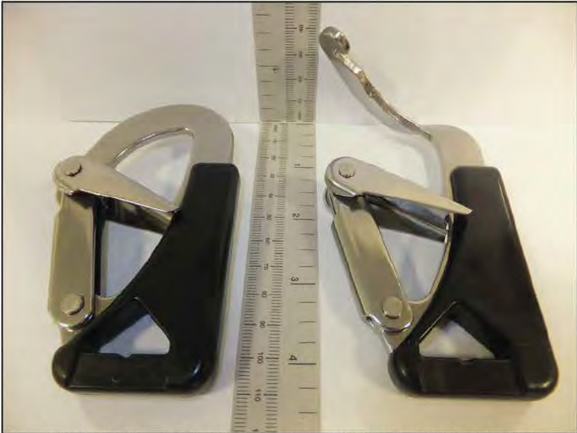
Figure 2: Example of a tether hook and a tether hook after lateral loading
