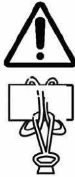
Figure 7 - Pictogram indicating correct attachment to multiple rings or points of attachment
