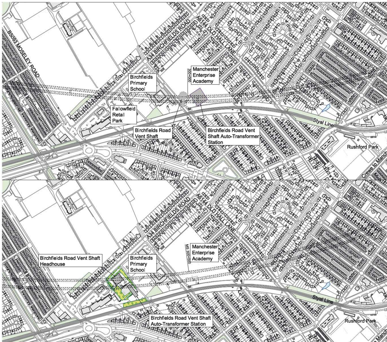
Figure 4: Plan showing the current design and proposed relocation of the vent shaft. For more detail see change two in Volume 2: Map book and visualisations.
