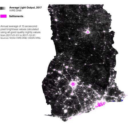
Because the radiance values are heavily right-skewed (i.e., there are some extremely large positive values, relative to the average), and some are slightly negative due to onboard calibration (the technical minimum is -1.5), I follow NOAA and add 2.5 to the remaining values and calculate the natural logarithm of all radiance values. To generate annual estimates, the average of all good quality nightly values for each pixel in each calendar year is calculated.
