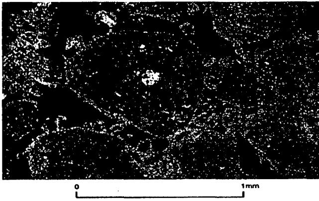
FIGURE 4 San Victor marl under crossed polar light, showing nucleation growth of one particle but nonnucleation in others; dark areas are voids.
