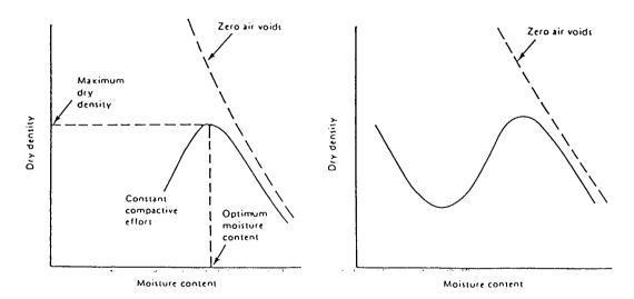
Fig. 1 Conventional compaction curve
