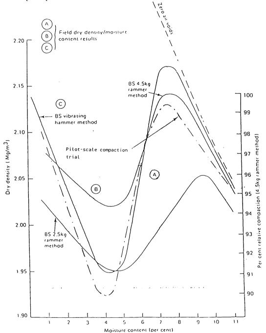
Fig 3. Laboratory CBR/dry density/moisture content relationship for road base gravel (full scale trial) with field results
