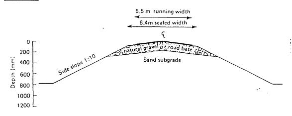
Fig 4. Layout of full scale trial in northern Kenya
