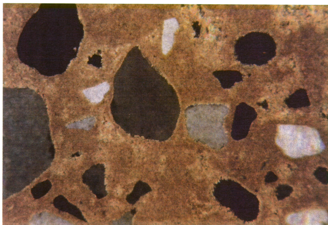
(d) MN2 Aggregate: sand particles in very fine grained (brown) calcite matrix. Photo taken under crossed polarised light.
