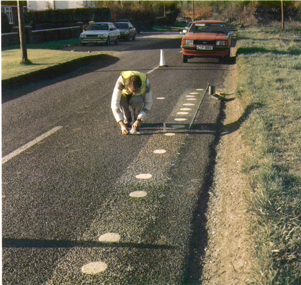
Plate 2 Measuring texture depth of trial panels by sand patch method
