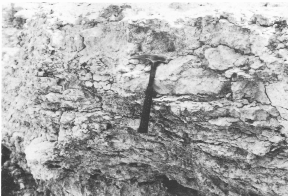
App. 2 Plate 4 Hardpan calcrete. The horizontal laminar structure is typical. The material grades downwards into tough powder calcrete at the bottom of the photograph
