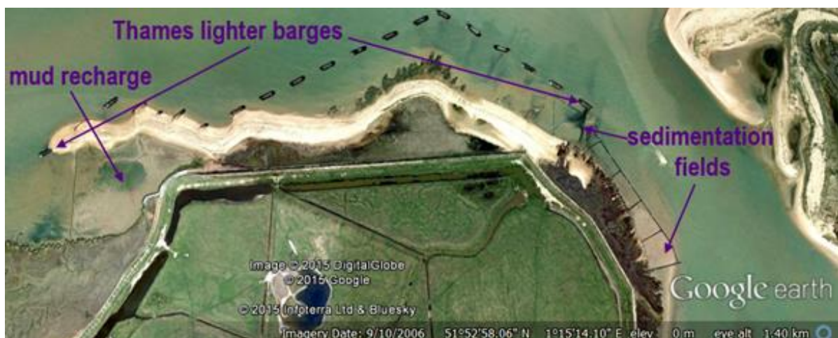
Figure 6: Image of Horsesey Island (north shore), showing recharge area, wave breaks, and sedimentation fields.
