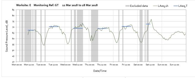
Note – Missing data between 03:00 on Saturday 10<sup>th</sup> and 11:00 on Monday 12<sup>th</sup> due to a pause in the measurement to enable changing the measurement configuration.
