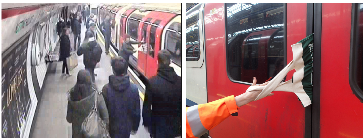
Figure 7: Image from station security camera (left) and RAIB reconstruction (right) showing the bag trapped in the doors
