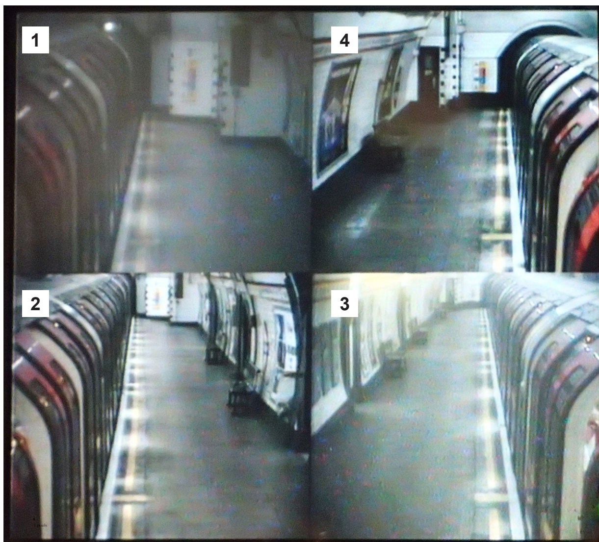
Figure 5: Typical arrangement of in-cab platform CCTV images on the Central line (numbers denote the ordering of images from front to rear of the train)
