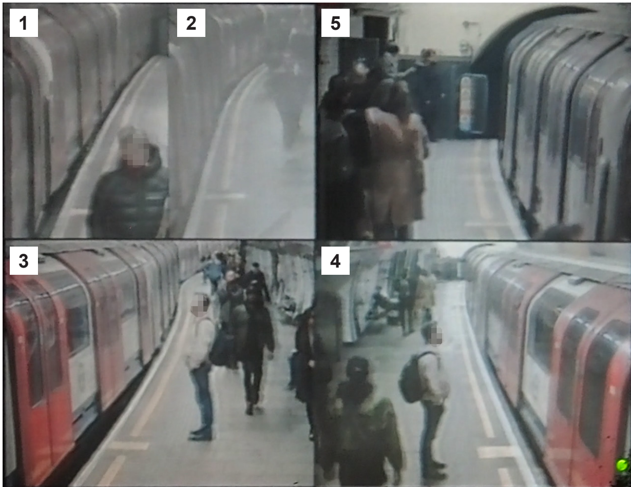
Figure 6: Arrangement of in-cab platform CCTV images at Notting Hill Gate platform 4 (numbers denote the ordering of images from front to rear of the train)
