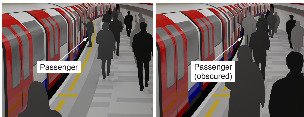
Figure 8: Virtual model of the perspective from the relevant platform-train interface camera showing the view seven seconds before departure (left image) and one second before departure (right image). NB: these represent the image that would have been displayed in the lower-left quadrant of the train operator's in-cab monitor.
