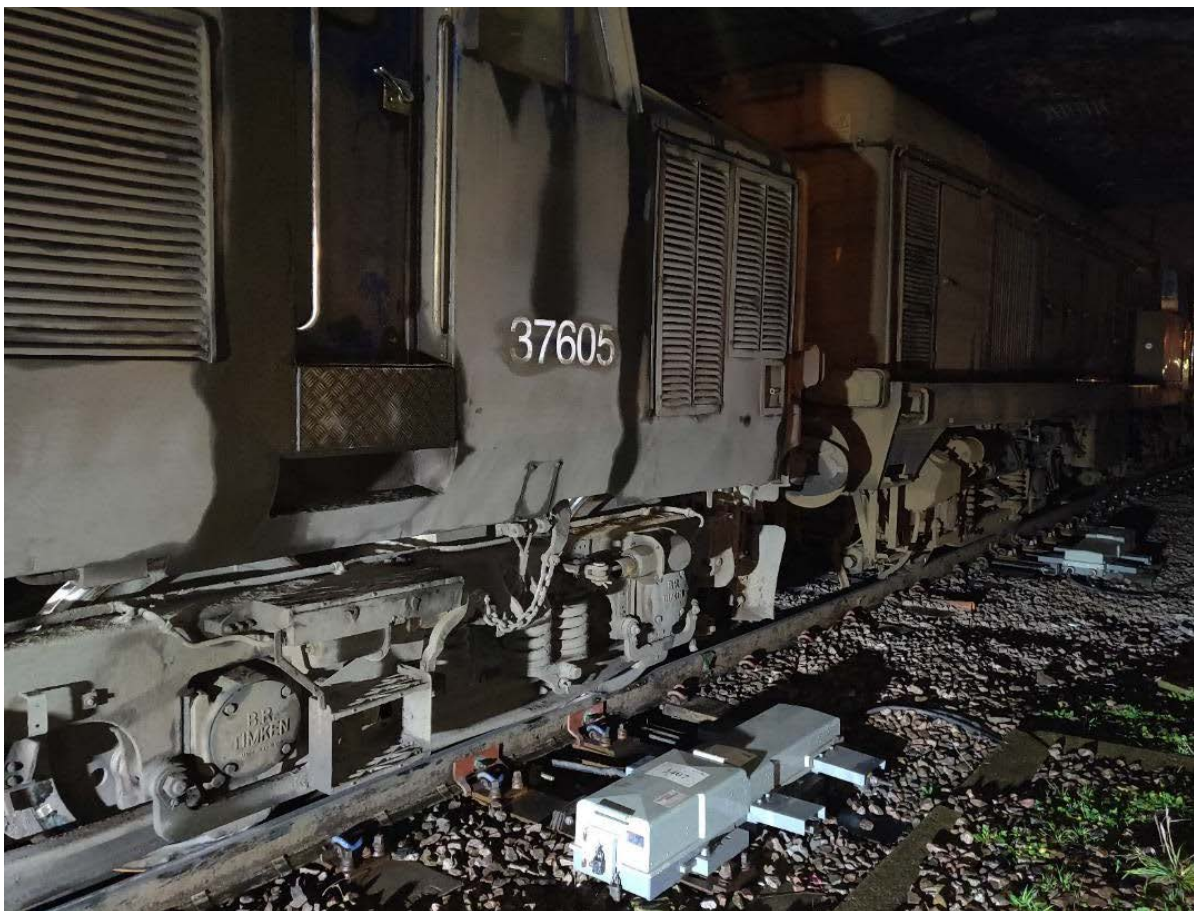
The Class 37 locomotive involved, with the second wheelset of its front bogie derailed
