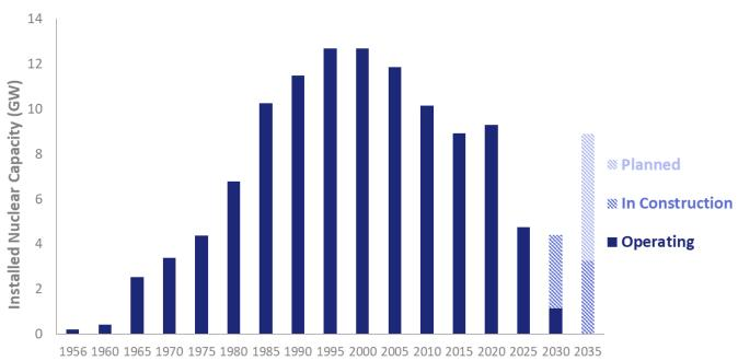
In 1956, Calder Hall opened in the UK as the world's first commercial nuclear power station and began to supply nuclear electricity to the public supply grid for the first time. This was a small-scale Magnox reactor, a design which was progressively scaled up and optimised, as 10 further Magnox power stations were opened in the subsequent 15 years. The design life of these reactors was
