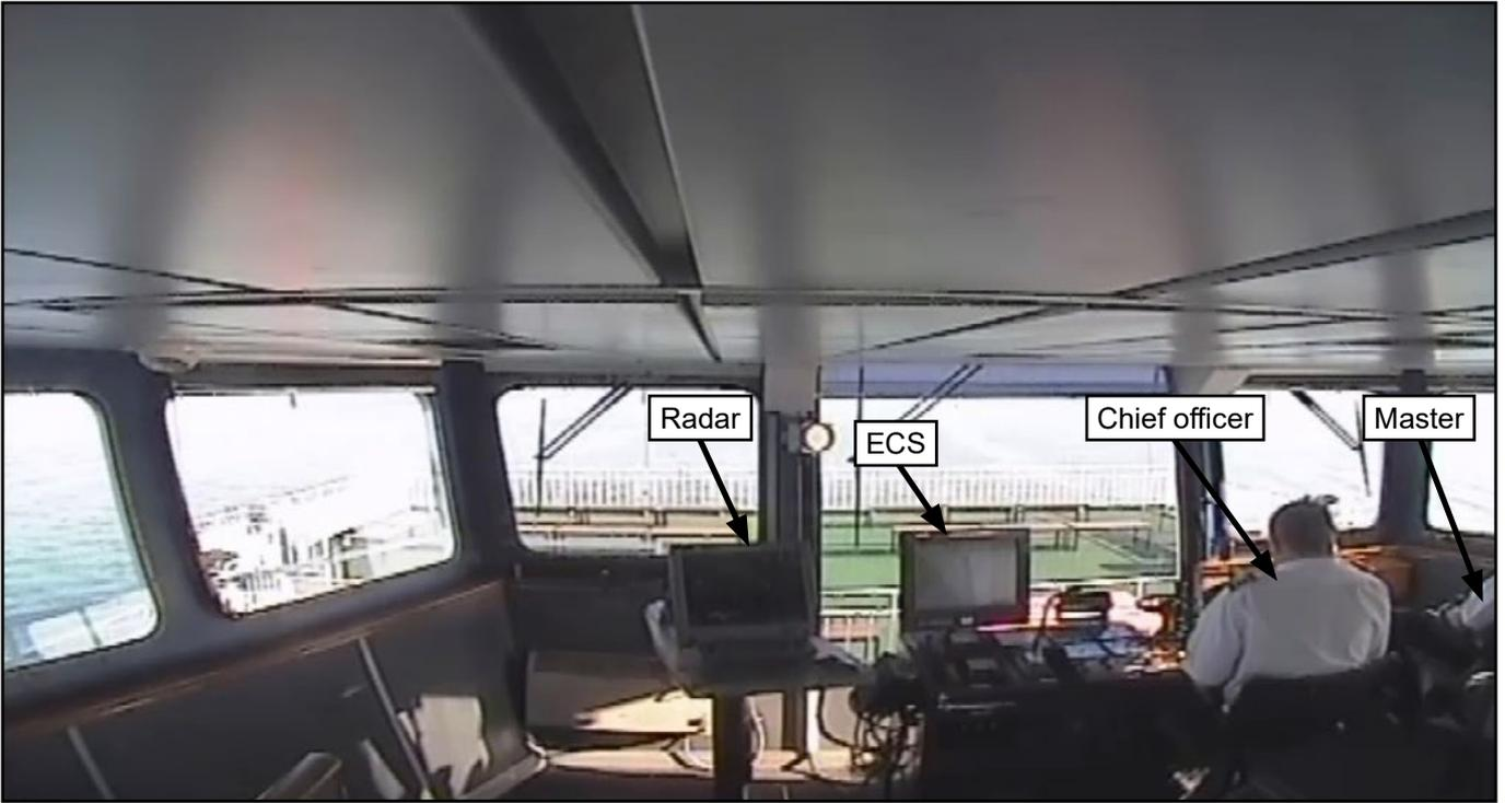
**Figure 2:** Red Falcon's bridge at 1627 (CCTV image)
