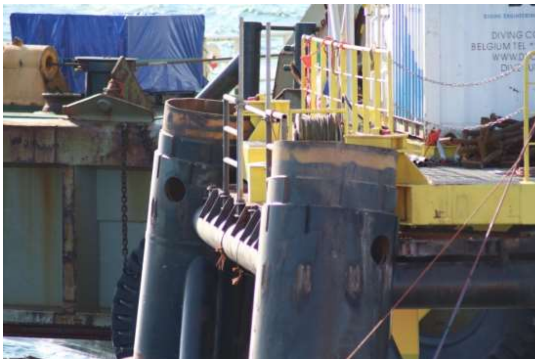
Photo 12 – Holes cut for lifting pins (July 2017)
