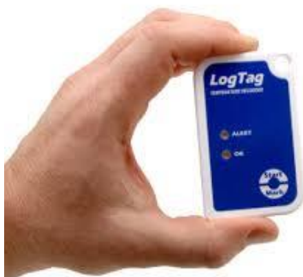
Figure B3 - LogTag temperature and humidity monitor
