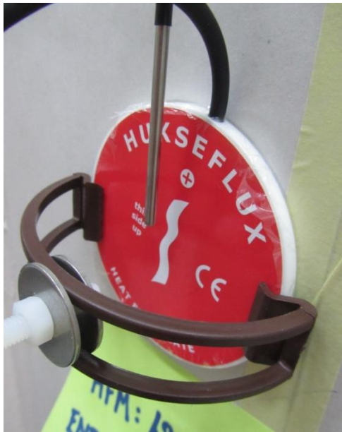
Figure 11: Thermistor sensor (metal-tube) mounted close to the HFP surface
