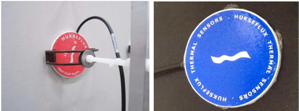
Figure 5 - Image of a HFP pressure-fixed to the plasterboard surface of the test panel and image of the underside of the sensor when removed
