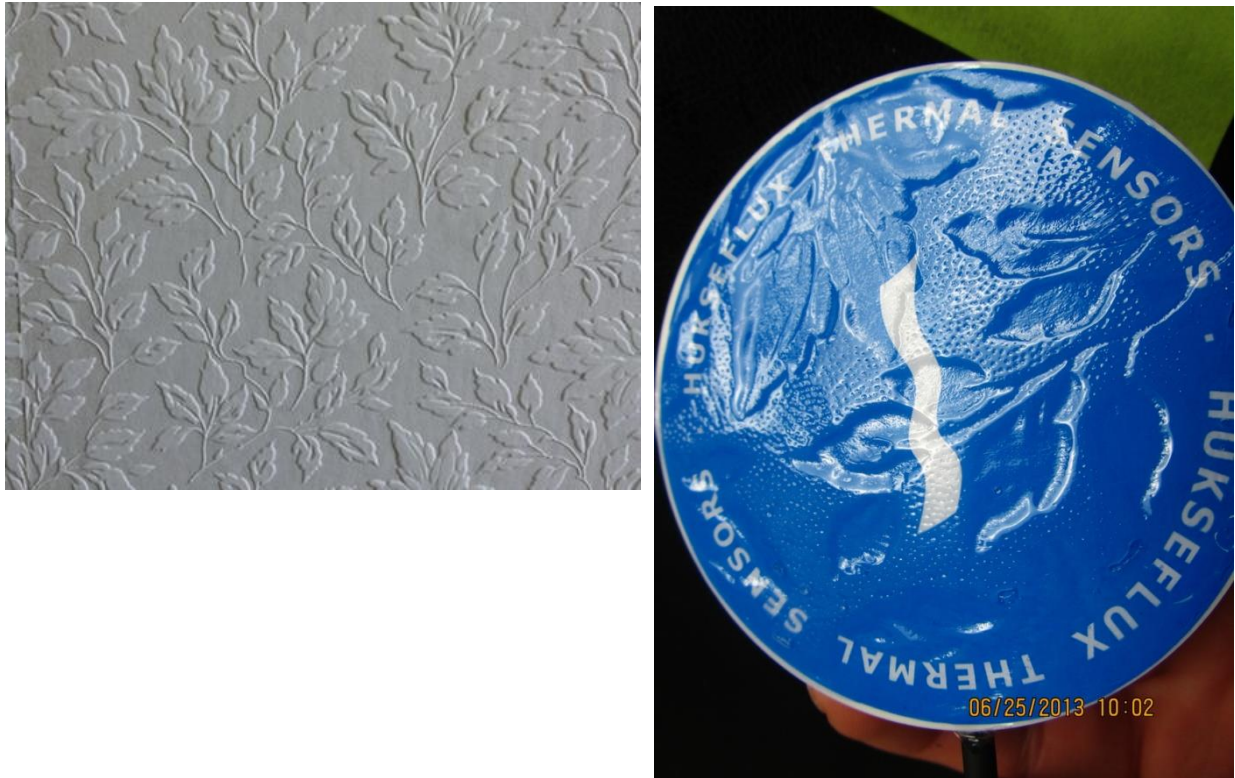
Figure 7 - Image close-up of embossed wallpapered surface of the test panel for Runs 4 and 5 and an image of the underside of the HFP after removal
