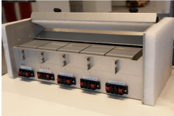
Figure 16 - Hukseflux Calibration apparatus showing locations for up to five HFP to be calibrated
