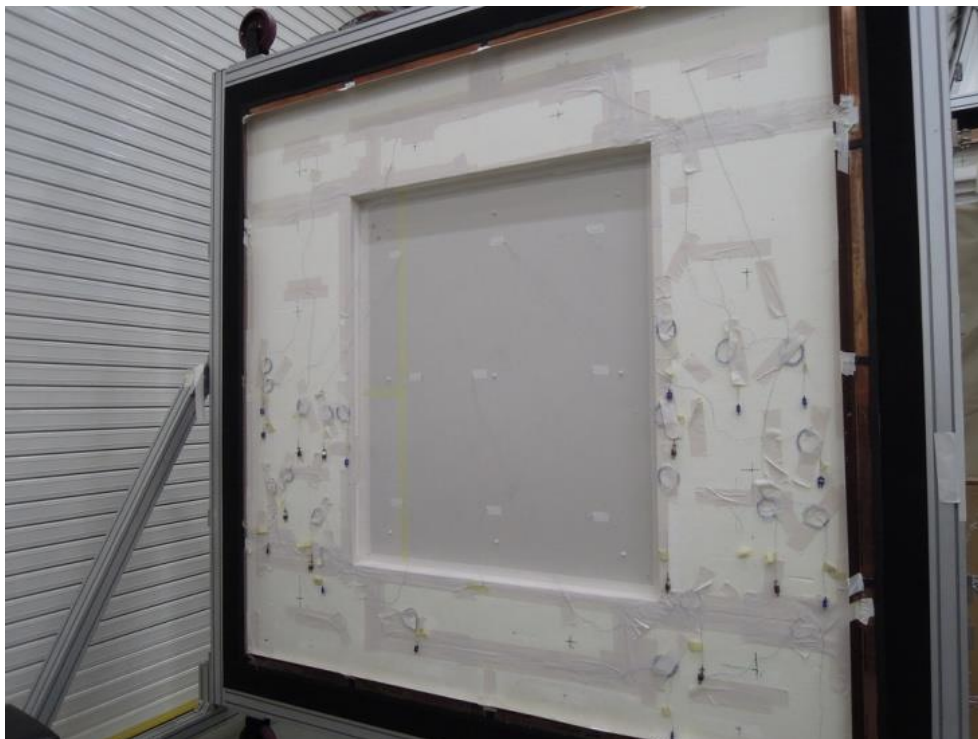
Figure 1 - 'Cold-side' of NPL hot-box test element showing the inserted test panel
