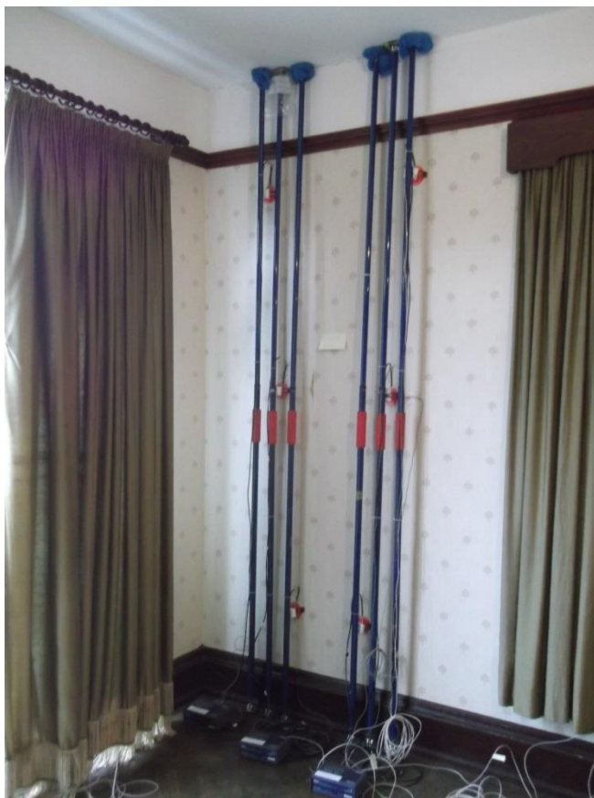
Figure 36 - Vertical stratification test setup
