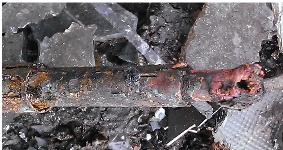
Figure 12: Example of DC connector contact that has been subject to electrical arcing. The right hand end has been melted.
