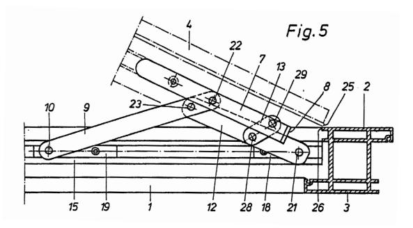
22. At the carrier arm 12, at a predetermined distance from the hinge point 21 of the carrier arm 12 one end of a guide rod 13 is hinged to the sliding part 18 at 28, the other end being hinged to the casement mounting plate 7. The open position of the casement 4 is determined by the abutment of the sliding part 18 at a stop part 19 which is secured to the guide rail 15 and may also bear the pivot bearing 10 for the scissor arm 9.
