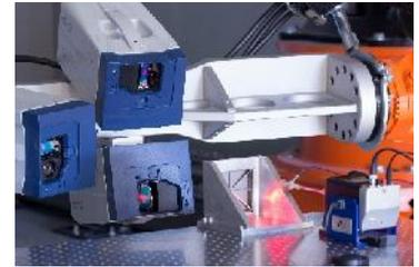
It has been used for upstream space projects, especially in structural and vibration analysis of payload mechanical designs. 3D laser Doppler vibrometry (LDV) is ideal for measuring the structural dynamic properties of lightweight materials. Thin films used in detectors, optics and deployed arrays can only be tested using LDV.
