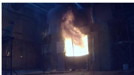
40 minutes (frame above sill falls away)
