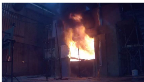
40 minutes (frame above sill falls away)
