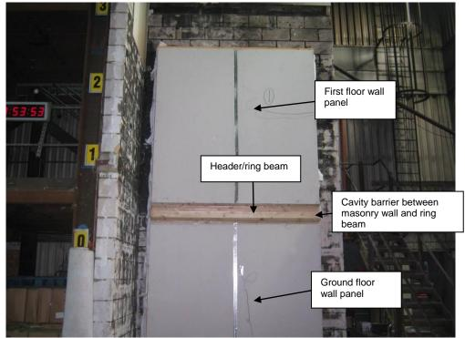
Figure 25 - Experimental set up for cavity barrier fire tests
