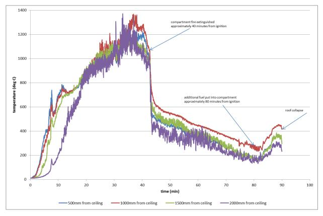
Figure 20 - Compartment temperatures (North West corner)
