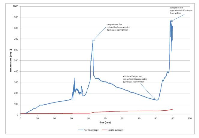
Figure 21 - Average temperatures in roof void either side of compartment wall
