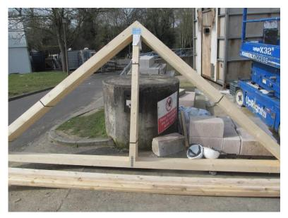
Figure 13 - Trussed rafters used for compartmentation in roof voids experiment
