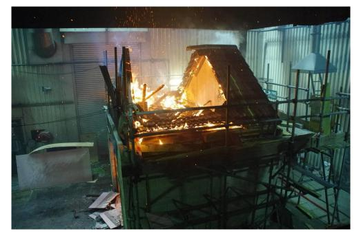
Figure 22 - Collapse of roof structure with compartmentation intact
