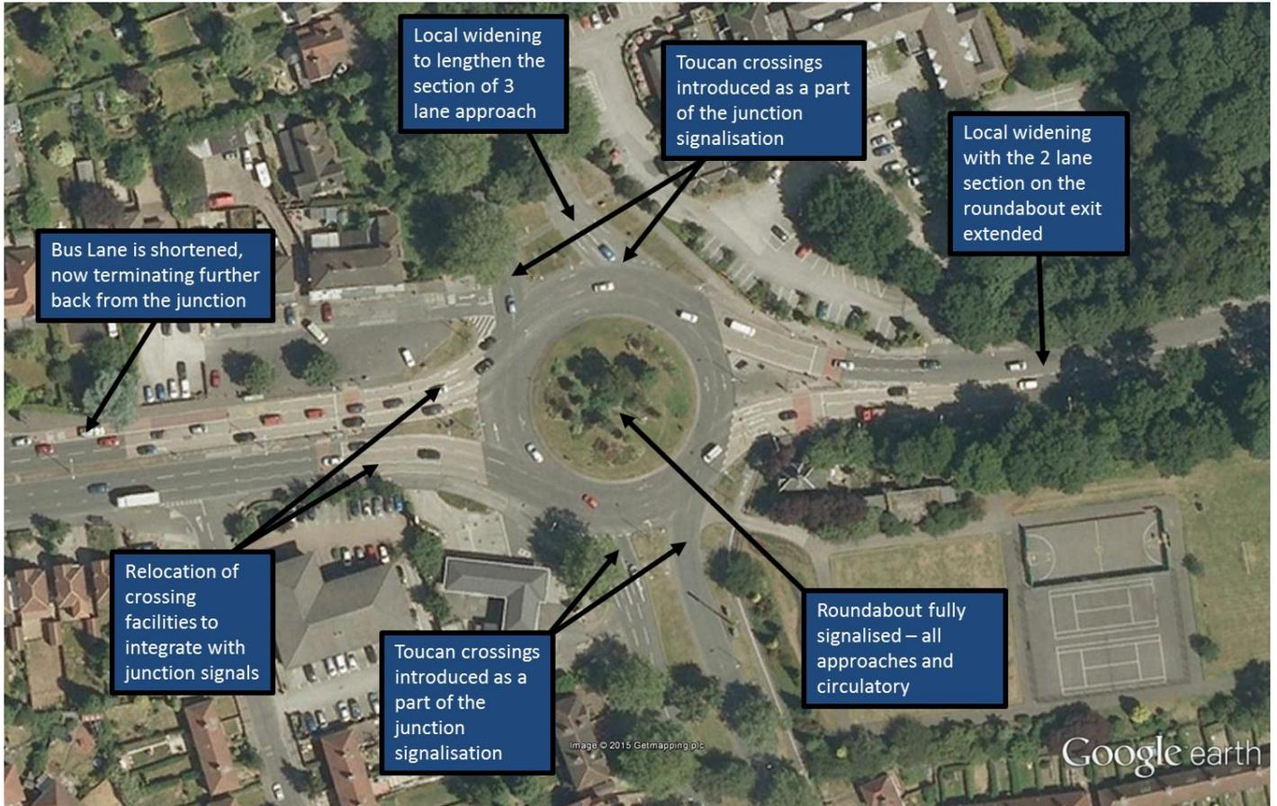
**Figure 2.5 – QMC Roundabout: Scheme Measures**
