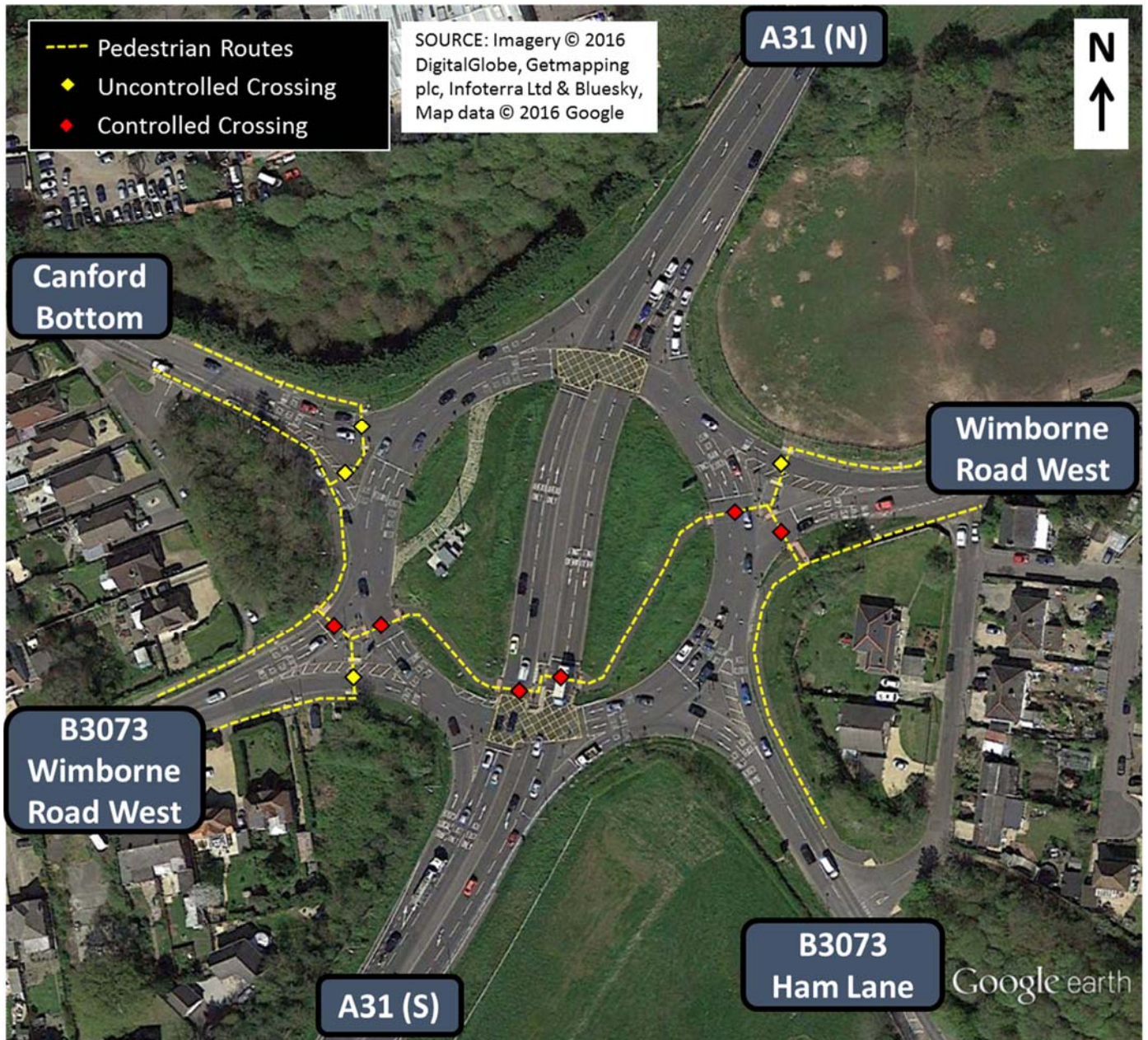
Figure 2.3 – Post-Scheme Junction Layout
