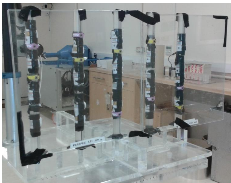
Figure 2: Dosimeters prior to the ^{137}\text{Cs} exposure, with PMMA build-up in front of the dosimeters mounted on rod phantoms.
