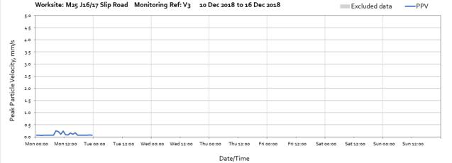
Note – Missing data from 00:00 on Tuesday 11<sup>th</sup> due to a technical fault of the vibration monitor. The instrument was returned to the manufacturer, and a replacement monitor was installed at the same location on Thursday 20<sup>th</sup>.
