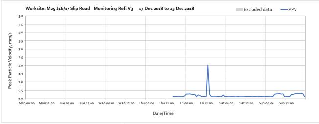
Note – Missing data from 00:00 on Tuesday 11<sup>th</sup> due to a technical fault of the vibration monitor. The instrument was returned to the manufacturer, and a replacement monitor was installed at the same location on Thursday 20<sup>th</sup>.
