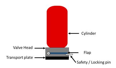
Figure 1 – Typical Explosion Suppressor Valve Head Assembly Schematic
