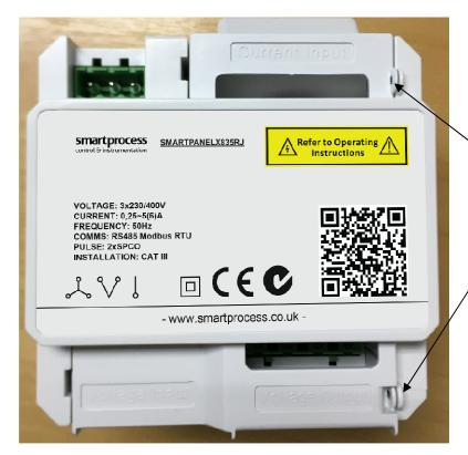
RJ45 Terminal cover sealing point
