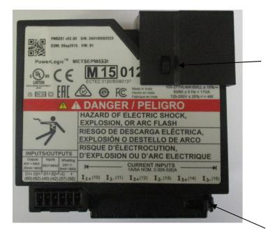
Voltage Terminal Cover Sealing Point
