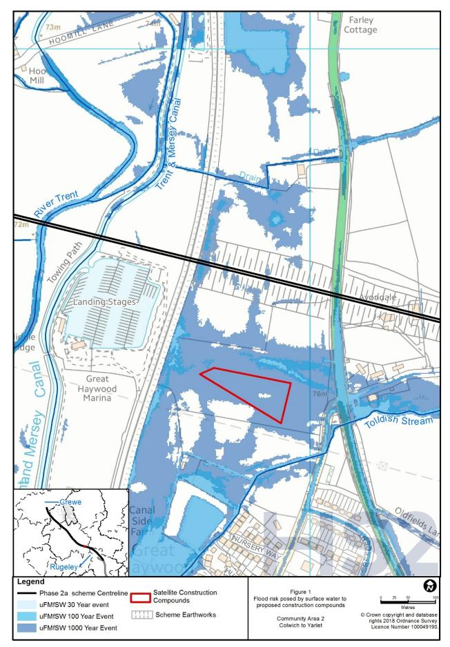
Figure 1: Surface water flood risk to the proposed temporary construction compound
