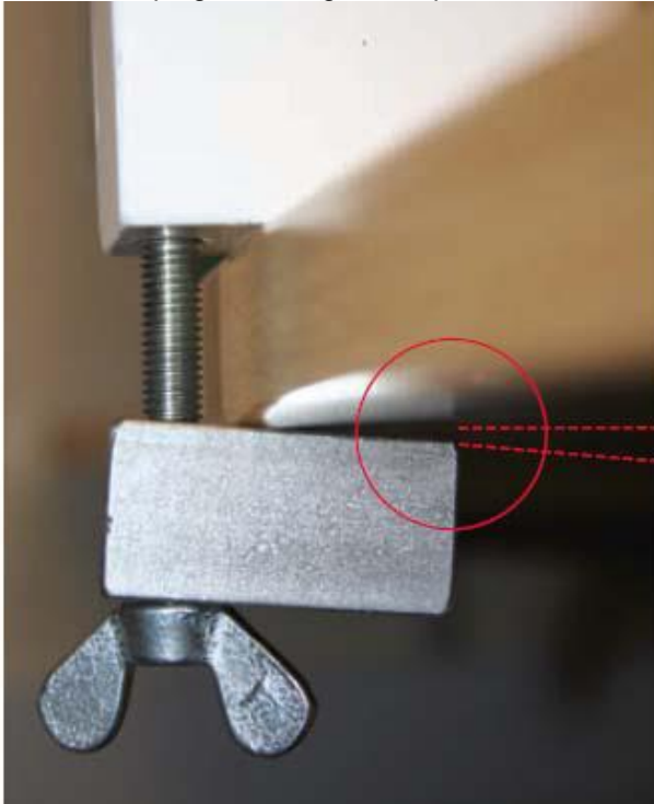
Pic 3: Clamping bar being used upside down
