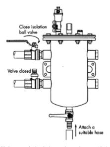
Attach a suitable hasing method to the bottom drain valve to enable the draining of the fluid in the filter pot housing.
