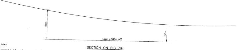
Horizontal distance between anchors is approx 1237m
