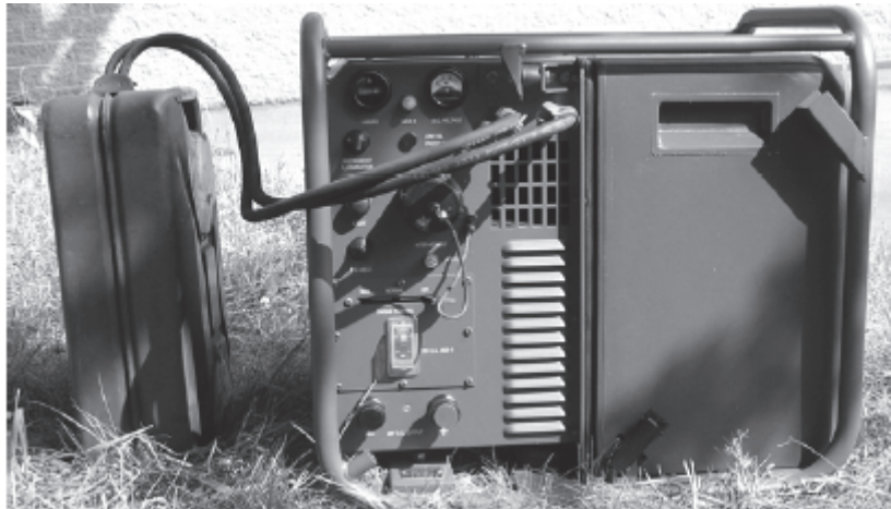
Fig 5 Jerrycan connected to fuel quick disconnected couplings
