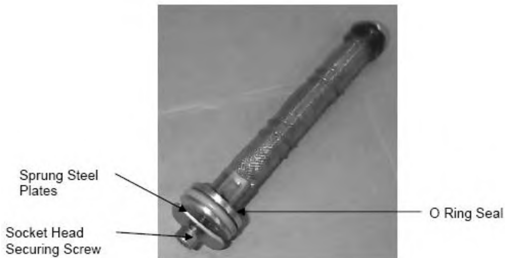
Fig 12 Oil filter strainer assembly
