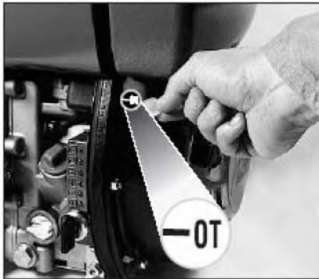
Fig 31 Flywheel cover inspection hole
