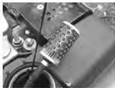
Figure 8 Engine Fuel Tank Fuel Filter
