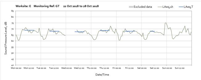
Note – Missing data between 00:00 and 10:00 on Wednesday 24 due to sound level meter failure.
