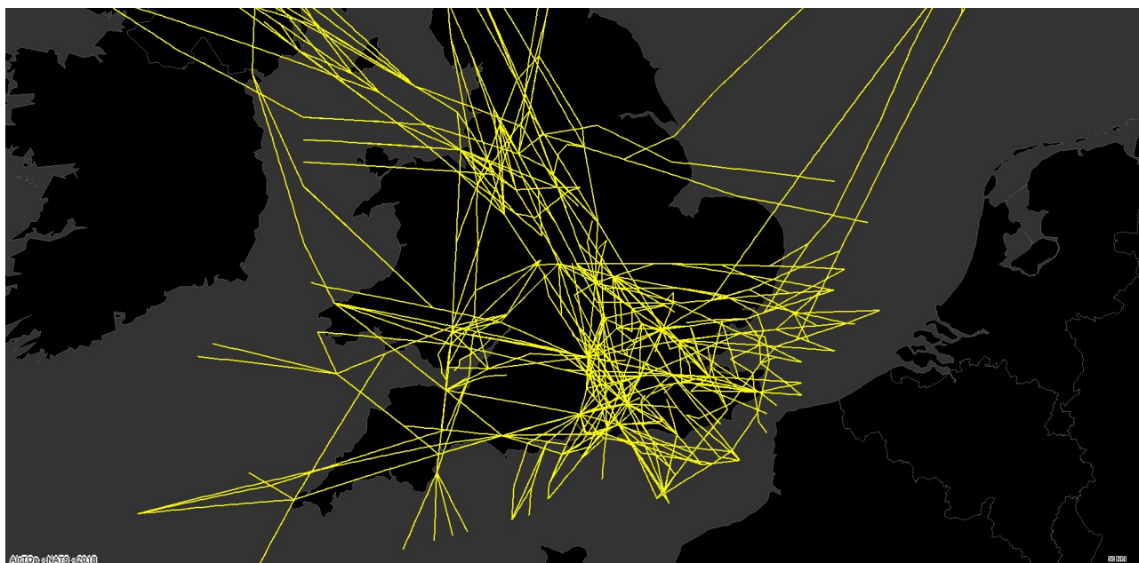
Figure 1: The current route structure for the 15 airfields in the FASI-S programme (largely based on historic VOR locations).
