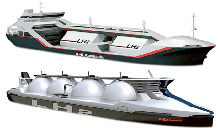
SHIPS being built and planned by Kawasaki Heavy Industries to carry liquid hydrogen extracted from Victoria's brown coal could one day be operating out of the Port of Hastings. The top "test" vessel will carry 2500 cubic metres of liquid hydrogen and the larger vessel, below, is designed for 160,000 cubic metres.
