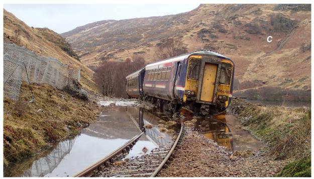
Figure 3: Front view of derailed train. Another recent landslip is visible in the distance on the opposite side of Loch Eilt (marked 'C').
