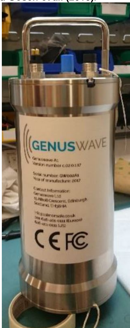
Figure 2.10 Example of the fully submersible prototype ADD pod currently being developed by Genuswave Ltd.
