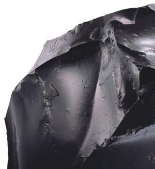
Example of products generated from alternative treatment processes thermal (left) and geopolymers (right) (Both images courtesy of the National Nuclear laboratory)
