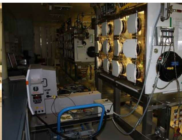
Raman spectroscopy linked to a glovebox to analyse plutonium containing solids
