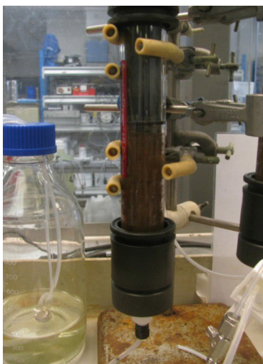
Column experiments at the University of Manchester to research techniques to control the spread of groundwater contamination
