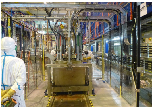
Research is ongoing into the feasibility of thermal treatment as a technique to immobilise wastes at Sellafield, this is a test facility in the NNL Workington facility. Cameras inside the melter provide the ability to monitor progress (Both images courtesy of the National Nuclear laboratory)
