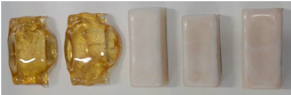
Research on glass formulations so that new feeds arising from wash-out operations during POCO may be successfully solidified by vitrification
