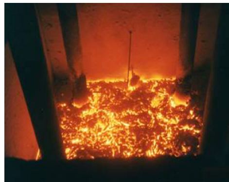
Research is ongoing into the feasibility of thermal treatment as a technique to immobilise wastes at Sellafield, this is a test facility in the NNL Workington facility. Cameras inside the melter provide the ability to monitor progress (Both images courtesy of the National Nuclear laboratory)
