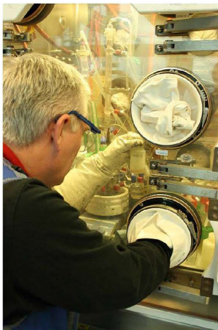
Operator working with a radiochemical glovebox (Image courtesy of the National Nuclear Laboratory)
